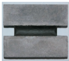
图1 标准填缝料试件 Fig. 1 Standard test specimen of joint sealant
