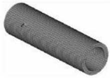
2 光滑试件及其网格划分 Fig.2 Finite element meshes for the smooth specimen
