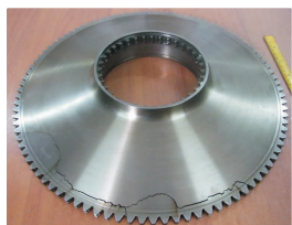
图 10 齿轮毂裂纹外观图 Fig. 10 External view of flaw for gear hub
